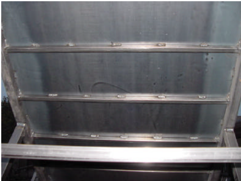
Figure 31 - I advise you to use 5 welds per Cross Support. On ramps I have built with only 3 or 4 welds per Cross Support, the ramp was noticeably nosier.
